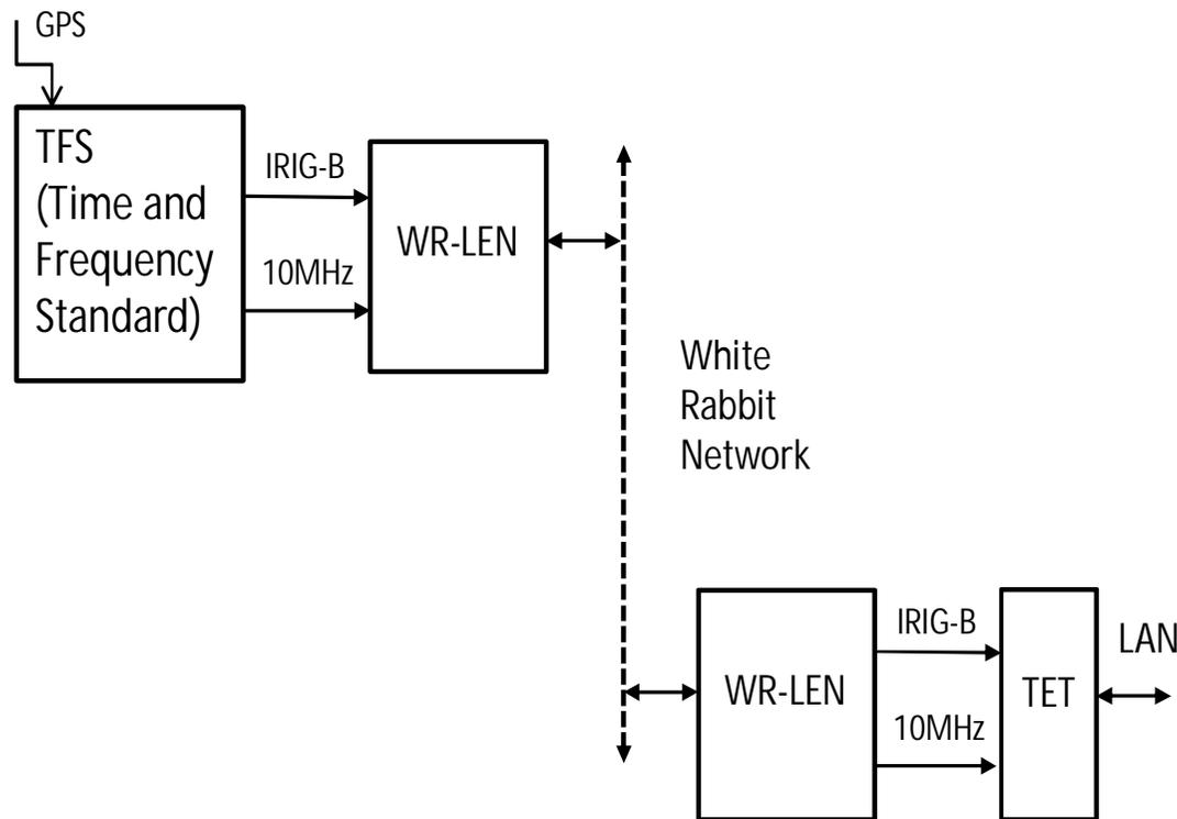
The on-board computer of the TET should work in a network server mode and provide data packets that contain time-tag information. The schematic of the TET has been captured and the PCB design has been done. It is planned to build a prototype in the spring this (2018) year. It is planned to use WR-LEN modules (Seven Solutions). As a TFS the GMR1000 (from MASTERCLOCK, Inc.) is planned to employ.
