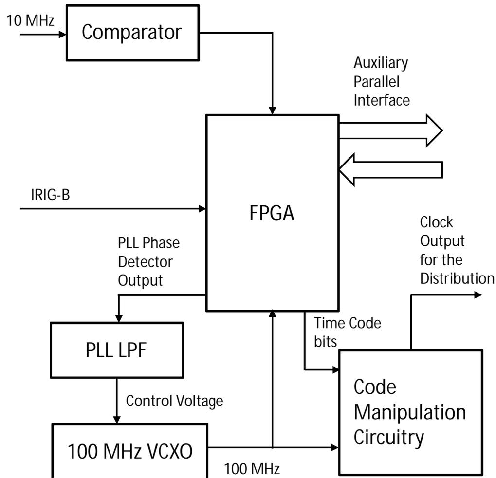
The Comparator performs the signal conditioning of the 10 MHz input signal (it could be a pulse or sinusoidal signal with different amplitude). The LVTTTL signal from the output of the Comparator comes to the FPGA.
