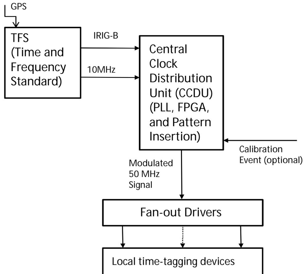
The operation of the system is based on the use of a TFS. The TFS produces a stable clock signal (10 MHz as a rule) alongside with the Time Code signal (IRIG-B standard is suggested to be used as one of most popular). Such device normally can be disciplined from the GPS network and is usually based on a Rubidium standard or a TCXO (temperature compensated crystal oscillator).
