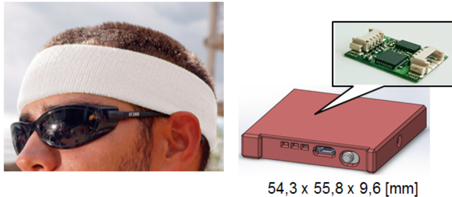
Figure 1.3.25: Sensor module for head position monitoring.
