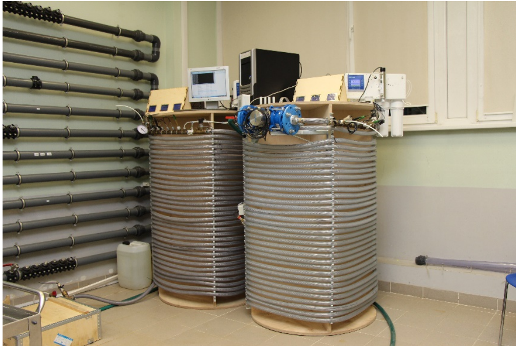
Figure 4.6.3: Lab-scale (pilot scale) DWDS.
