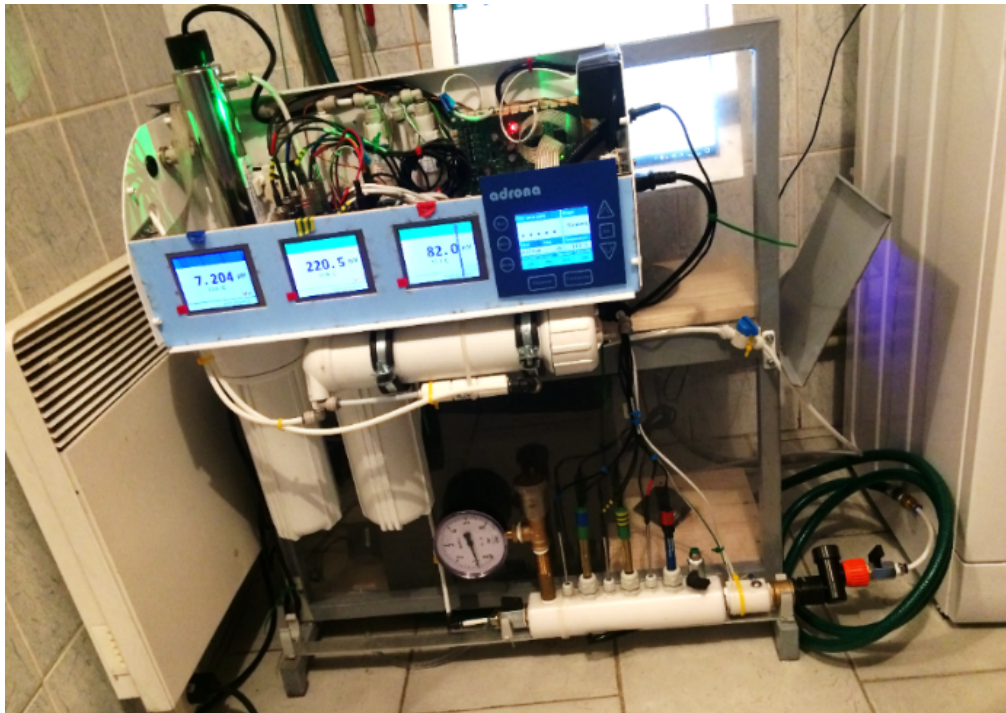
Figure 4.6.23: The drinking water quality monitoring system during approbation experiments.
