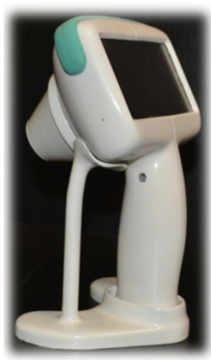
Figure: Sklmager earlier proposed skin assesment prototype, polarized illumination 5 LEDs, cross polarized CMOS Sensor
