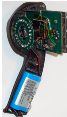
Figure: Sklmager earlier proposed skin assesment prototype, polarized illumination 5 LEDs, cross polarized CMOS Sensor
