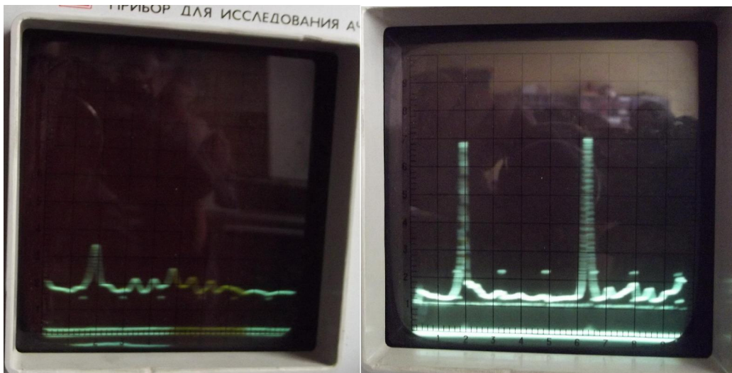
Figure 6.5 AFR of the rectangular patch resonators. Left – with conductive pigment. Right – with aluminum foil.
