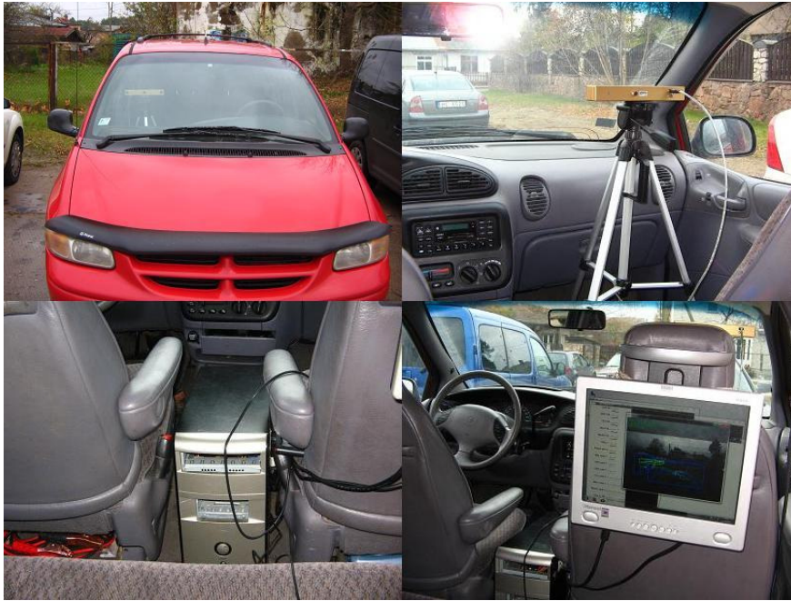
Figure 3.5 Setup of the test vehicle during approbation activities
