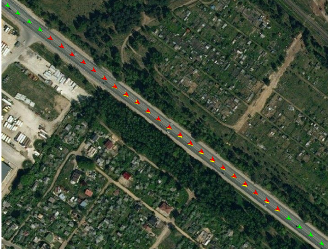
Figure 7.42 Position determination by using inertial sensors data with bias filtration
