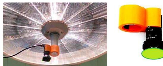
Fig. 2 The rPPG device attached to surgical lamp.
