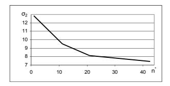
Fig. 3. Dependence of  $\sigma_2$  from the number of decimations between the selections using udc method, in  $\mu V$ .
