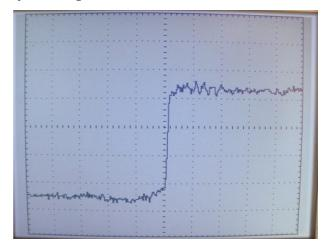
**Fig. 2.** The result of conversion of 200  $\mu$ V voltage stap with the *udc* method. For averaging every 42<sup>nd</sup> selection of the *ud* procedure is taken, output noise  $\sigma_2 = 7.4 \mu V$ .
