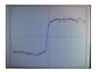
**Fig. 1.** The result of conversion of  $200\mu V$  voltage step with the *udc* method. For averaging all selections in succession are taken, output noise  $\sigma_2 = 12.8 \mu V$ .
