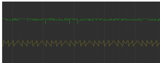
Figure 3.13: 2HZ, 2mV saw tooth signal after digitization, Green - CH1. Yellow - CH2
