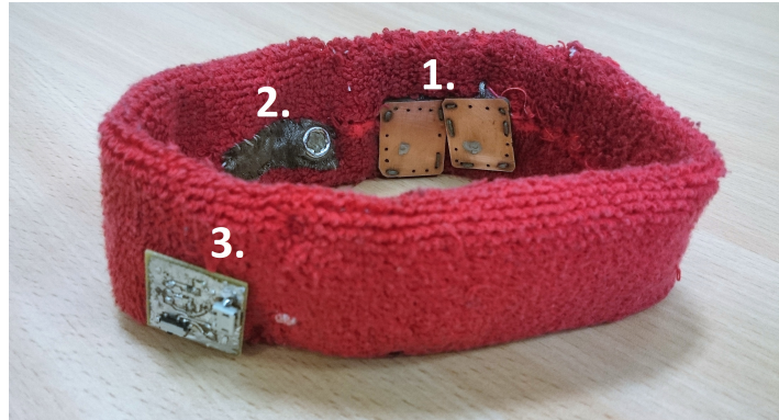
Figure 3.31: Wireless headband prototype with (1) dry-contact electrodes, (2) reference electrode, (3) charging port
