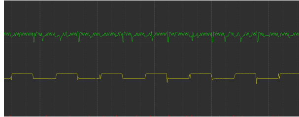
Figure 3.12: 1kHz, 50mV square signal after digitization, ADS is reconfigured. Green - CH1. Yellow - CH2
