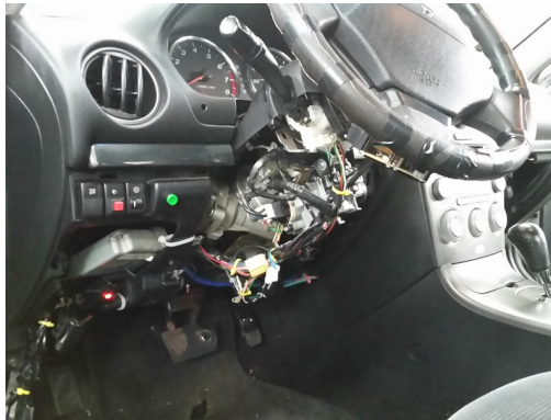
Figure 1.4.6: Electric Power Assisted Steering motor assembled in Mazda 6 steering column
