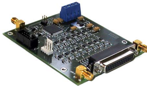
Figure 6.11 Pilot design version of the 16-channel data acquisition system module performing analog-to-event conversions
