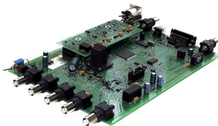
Figure 6.9 Pilot design version of the event-timing system
