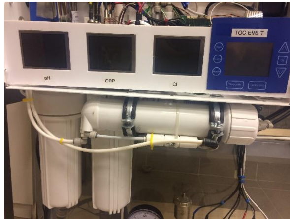
Figure 4. Ultrafiltration membrane and ion exchange resin for TOC measurements
