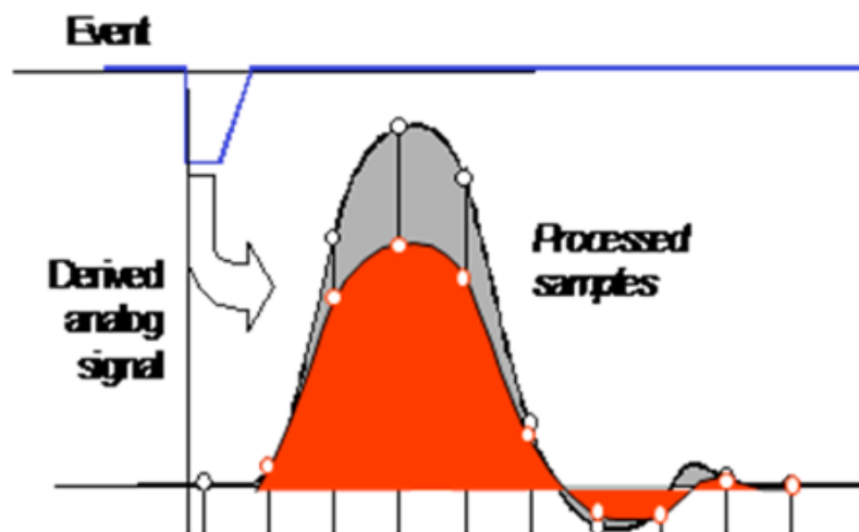
Fig.1.16. A temperature distortion of the event derived analog signal.
