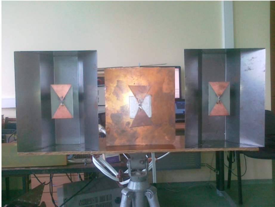
Fig. 2.4.1 Optimal reflector of antenna
