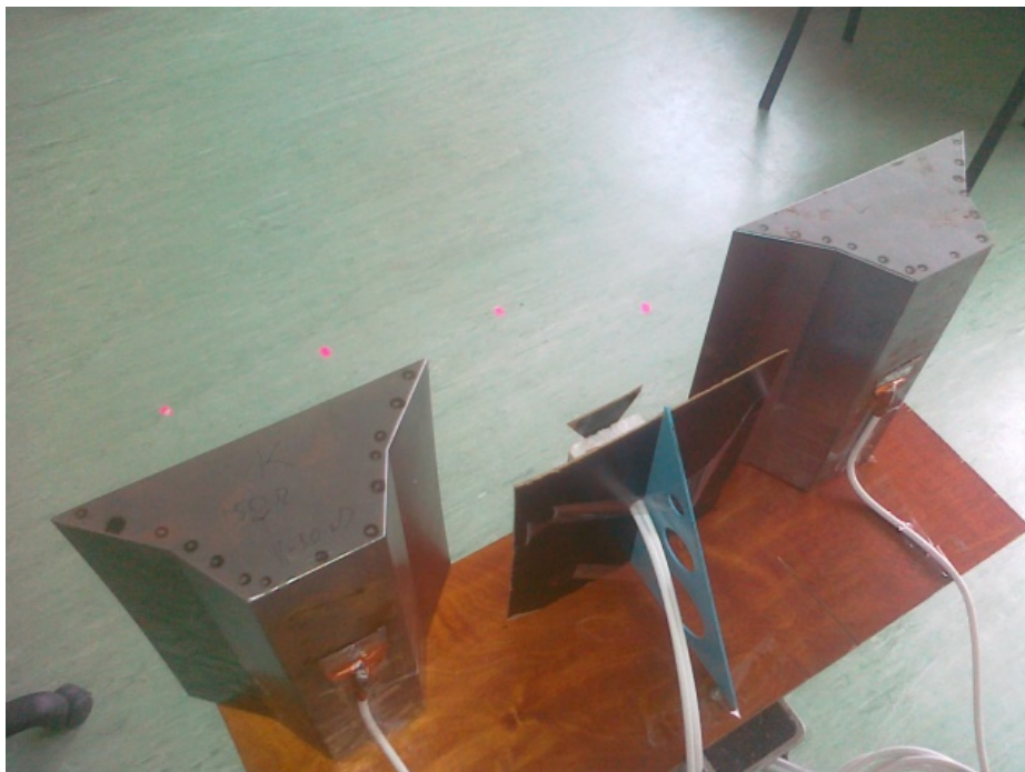
Fig. 2.4.2. Optimal reflector of antenna top view
