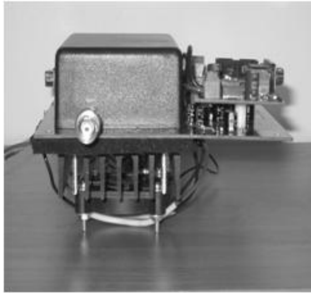
Fig.1.15. Event timer module with the measurement node placing in the thermostat with cooling on the base of Peltier elements
