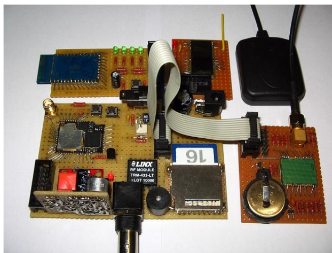
Figure 3.4 First prototype of the CarMote embedded device
