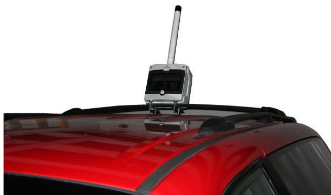
Figure 3.2 First mobile vehicle unit prototype
