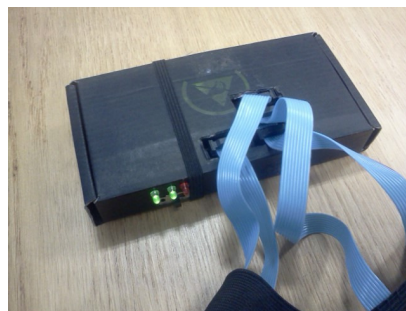
Figure 4.4 Enclosure protecting the central processing module and Bluetooth module
