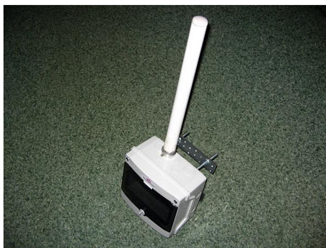
Figure 3.3 First stationary road side unit prototype
