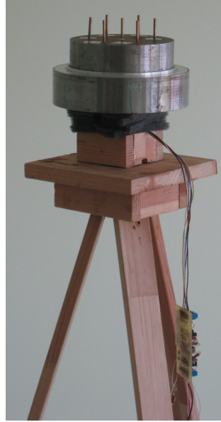
Fig. 2.1.3.2.2. Our Antenna testbed allows rotating the antenna in 360°.
