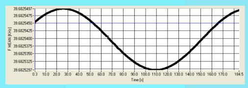
Min = 39682.53 Hz, Max = 39682.55 Hz, Pkp = 0.02 Hz, Mean = 39682.54 Hz,
