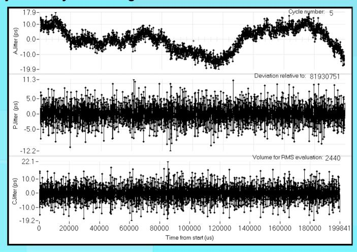
Single-shot measurement with picosecond resolution Simultaneous determination of multiple jitter characteristics
