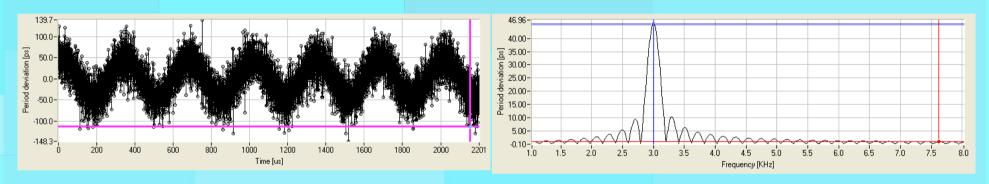
3.3 MHz carrier signal; 500 Hz deviation (period deviation - 45.9ps)
