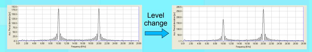
3.3 MHz signal with 28 Hz frequency deviation (modulation frequency 10 KHz) + 1% AM depth (modulation frequency 20KHz)
