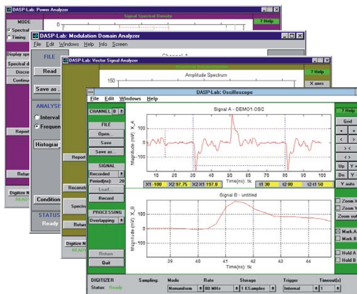
Figure 4. Instrument panels of DASP-Lab system programmed in MATLAB.
