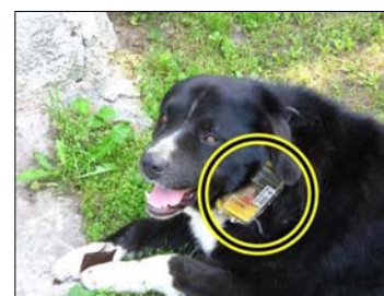
MansOS used for lynx monitoring: mote attached to "experimental lynx"
