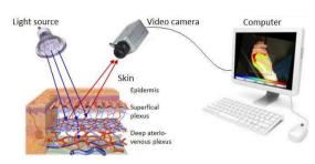
Fig. 1 The principle of rPPG technique.
