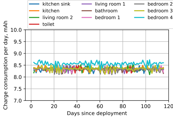
Fig. 11. Charge consumption history in a representative deployment (House 32) , software-based estimation. All nodes show stable consumption over time with only minor random variations, allowing to accurately predict the total software-estimated energy consumption.
