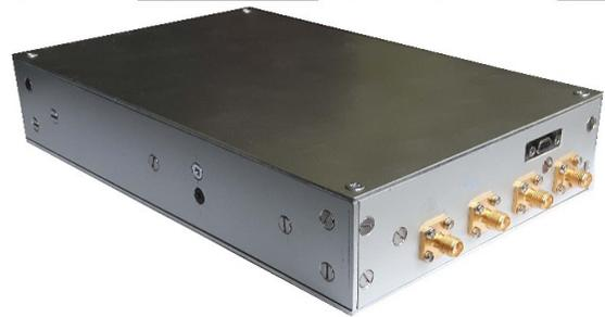
Thermal cycling test procedure in the range from  $-35^{\circ}\text{C}$  up to  $+75^{\circ}\text{C}$  at full MPET functionality revealed no any failures.
