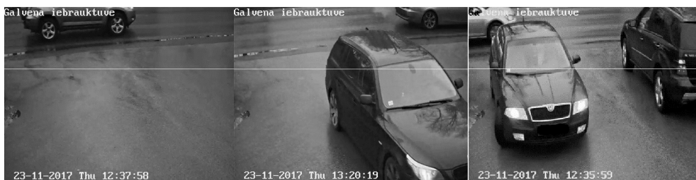
Fig. 1. (a) Video frame without vehicle; (b) Video frame with one vehicle on VDL; (c) Video frame with two vehicles on VDL.
