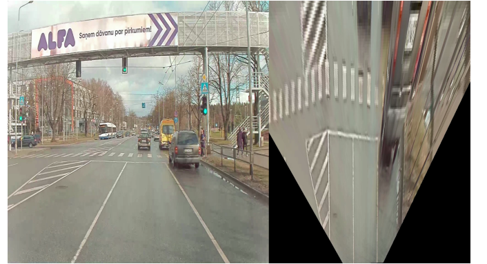
Fig. 6. BEV image (right) acquired using the proposed geometrical IPM approach on camera image taken on a EDI DbW Car test drive in Teika, Riga, Latvia (left)
