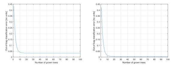
**Figure 3.** The effect of decreasing the number of trees on the accuracy of the Stage 1 classifier (**left**) and Sedentary classifier (**right**). 10 trees is a reasonable compromise between accuracy and feasibility for on-board implementation.
