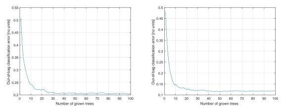
**Figure 4.** The effect of decreasing the number of trees on the accuracy of the Moderate classifier (**left**) and Rigorous classifier (**right**). 10 trees is a reasonable compromise between accuracy and feasibility for on-board implementation.
