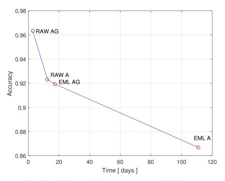
**Figure 5.** The trade-off between the model accuracy and lifetime. Legend: Raw Data—Accelerometer Only (RAW A); Raw Data—Accelerometer and Gyroscope (RAW AG); On-Board Classification—Accelerometer Only (EML A); On-Board Classification—Accelerometer and Gyroscope (EML AG).
