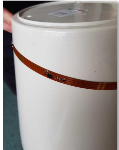
Picture 8: Sensor nodes on flexible PCB.
