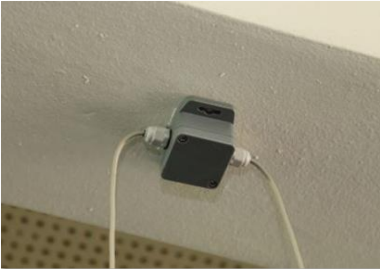
Picture 7: Sensor node in humidity resistant casing.
