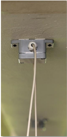
Picture 4: sensors installed on a crossbeam
