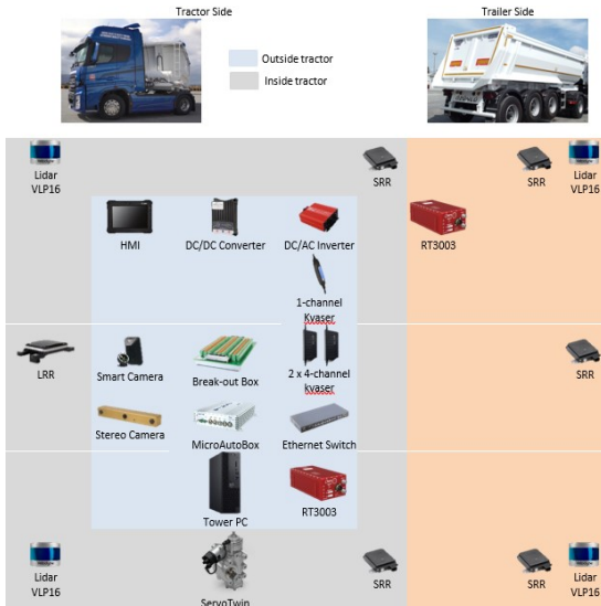
Fig. 27: Integrated hardware components on FORD HDV.
