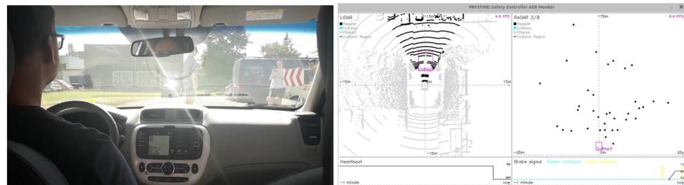
**Figure 7.** Snapshot of testing use-case with a pedestrian crossing the road without paying attention. Image on the right shows GUI (colours inverted) for the Aurix-based processing of LIDAR and RADAR data, heartbeat monitoring and break actuation.
