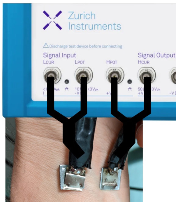
Fig. 3: Conceptual overview of the experimental setup with the electrodes and MFIA impedance analyzer.
