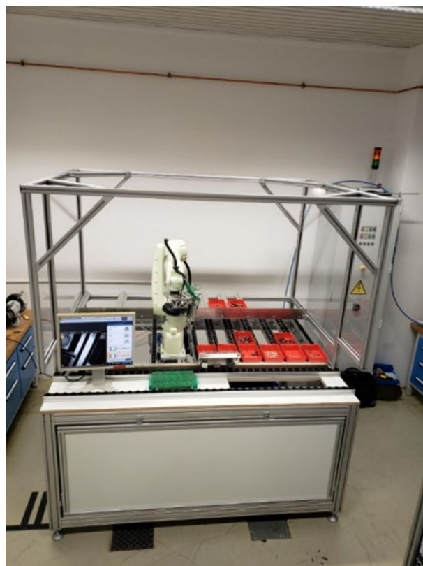
Figure 2. The assembly station for the automated THT-PCBs assembly.
