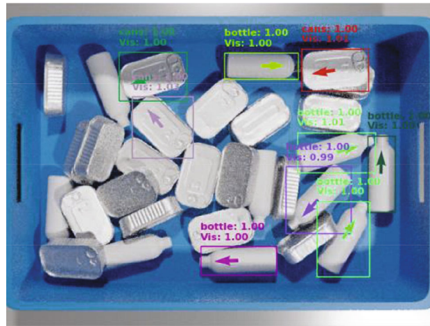
Fig. 7. DETR-POSE-2D output visualization with a class confidence threshold of 0.99 and visibility score threshold of 0.99.
